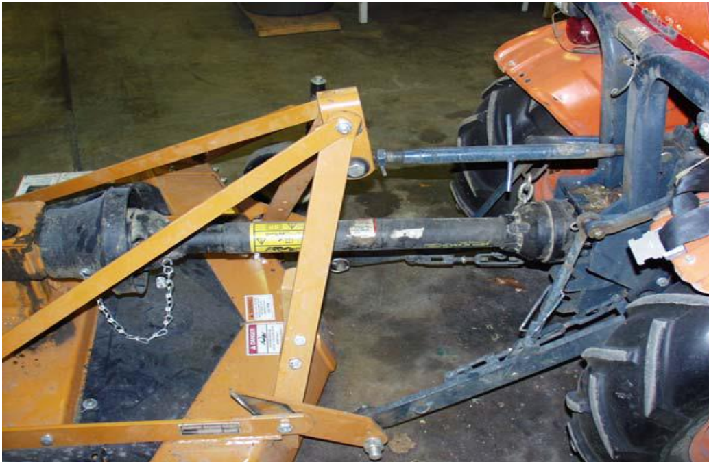
Figure 2.1 Tractor power take - off
